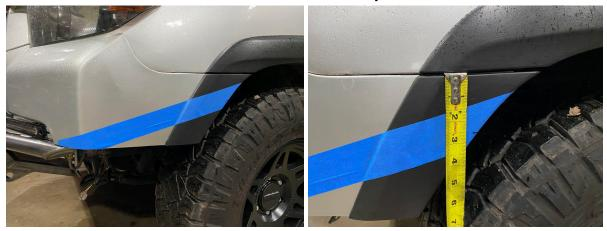
19) Use a flexible straight edge to draw a line from the outer wing of the bumper to the 2.5" mark on the edge of the wheel well.
