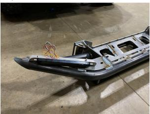
17) Using either a jack or two people, carefully lift the new bumper up to the vehicle so it is against the front frame plates. While holding it in place loosely install the inner M10 bolts with washers. Raise the new bumper till it is against the cut edge of the stock bumper. It is recommended to leave a 1/8" to 1/4" gap to prevent rubbing. There is also a little side to side adjustability. Once raised, tighten down the inner M10 bolts enough to hold the bumper.
