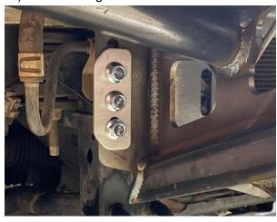
25) Adjust turn signal brackets and tighten hardware.
