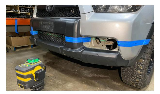
7) Undo any nuts / bolts / wiring attaching the stock plastic bumper to the vehicle and remove it. Or can leave it on the vehicle if desired, just make sure to not cut too deep behind the bumper and accidentally cut any wiring / fluid lines.
