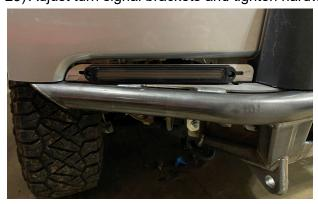
26) Install the lower aluminum cover using the 6x M8 flanged button bolts.
