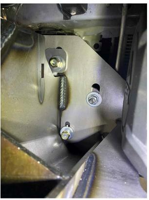
24) Adjust the bumper so there is an even gap and side to side spacing. Once height is set, tighten all hardware.
