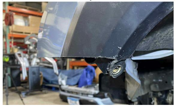
14) Cut wheel well liners. Can easily do this with a sharp knife.
