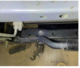
b) In the passenger side wheel well, undo the splash guard and remove the bolt holding the lines to the frame rail.
