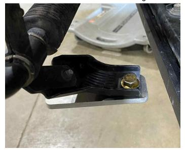
d) Loosely attach the offset brackets and coil to the crossmember using the longer hardware.
