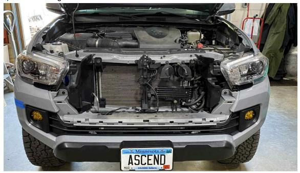
9) Unclip the ends of the fender flares from the bumper.
