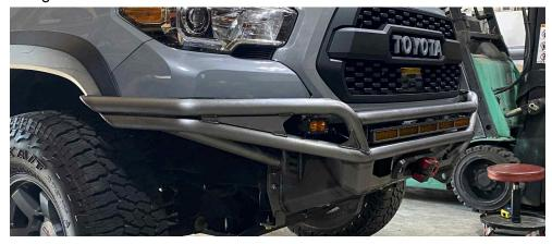
25) Install the lower aluminum cover using the M8 flanged button bolts. On uncoated orders you will receive both zinc plated and black stainless (for if you coat the skid yourself). If you ordered powdercoated you will only receive the black stainless hardware.
