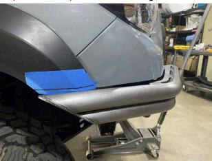
22) Install the inner M10 nuts and washers. Leave loose for now.
