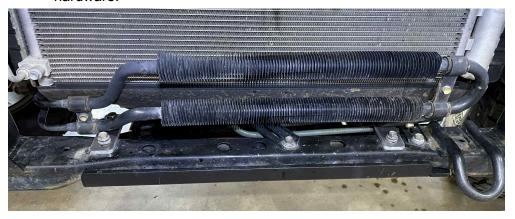
e) Using a long straight edge, hold it up against the plates on the ends of the frame rails. Make sure the coils are not touching the straight edge. Only need about 1/8" of clearance. Once spacing is set, tighten the hardware on the offset brackets and recheck spacing with the straight edge.
