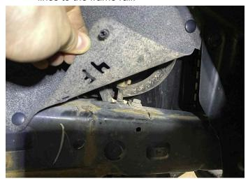
c) Loosely install the provided aluminum offset brackets. The coil feet should attach to the treaded holes on the brackets using the shorter bolts.
