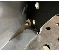
4. With the inner wing still clamped upside down to a weld table, take the outer wing and align the top edge with the edge on the inner wing. Start by aligning, clamping, and tacking the top edges of the wing. This should locate and correctly align the outer wing. Weld the inner top edge.
