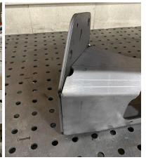
3. Put a small weld on the inside of the bumper along the mounting plate. Make sure to leave room for a bolt head.
