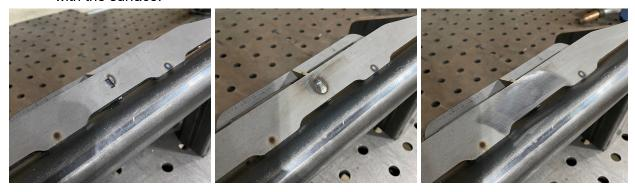
16. Weld along the edge of the top plate at each point where it meets the upper tube.
