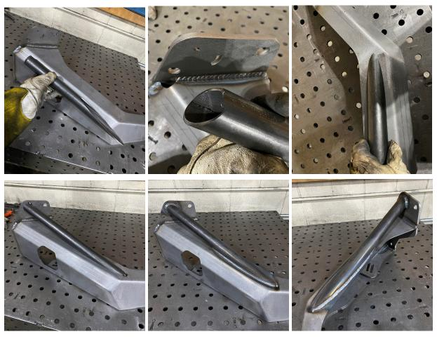
11. Lightly grind the edges of the mounting plates to knock down any weld that's hanging over the edges that could cause fitment issues with the cradle.
