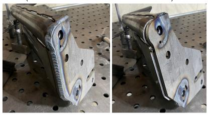
14. Fully weld the tabs on the top and bottom of the formed cover where they meet the tubes.
