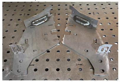
5. Using the two sub assemblies from previous steps, mounting plate, winch plate, and two winch plate supports, assemble as shown mating the tabs/slots between parts. Easiest method is to take the side sub assemblies, winch plate, and winch plate supports and hold them together using clamps/magnets over the mounting plate and drop all the tabs in at once.
