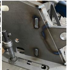
19. Weld the seam between the fairlead and winch plates.
