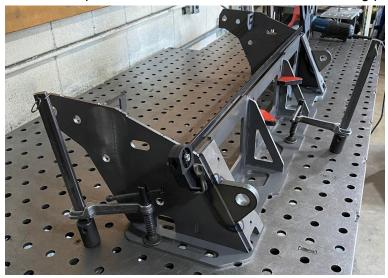
8. Put a small tack weld on either end of the side plates to the mounting plate. Put a large tack in the upper corner of the lower cover backing plate to the winch plate.
