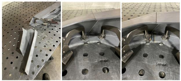
5. Clamp and tack around the rest of the outside of the joint between the inner and outer wings. Fully weld all exterior seams then grind smooth to a radius.
