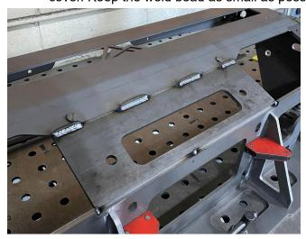
13. Weld over the tabs/slots on the front of the formed upper cover for the light brackets. Grind down welds so they are smooth and flush with the surface.
