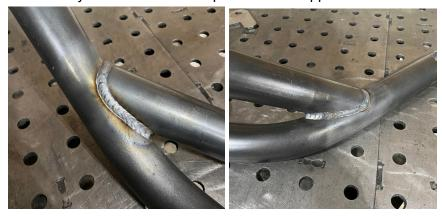
12. Align the formed cover so the edge meets up with the vertical edge on the mounting plate. Tack the upper and lower edges to the tubing.
