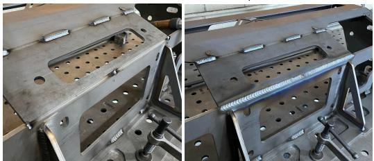
20. Weld the entire outer seams along the top and forward edges of the side plates between them and the formed upper cover, upper and lower cover backing plates, and the shackle mounts. (OPTIONAL: Weld the upper portion along the edge of the formed upper cover first and then grind the weld smooth to a radius. Then continue to weld the lower portion and leave the weld raw.)
