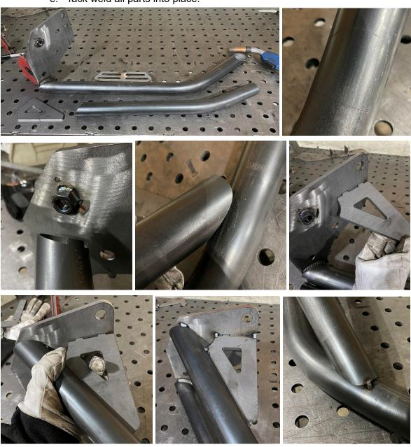
9. Fully weld the outer seams between the lower tube support, mounting plate, and lower tube.
