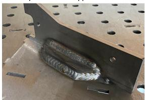
3. Take the light bracket and insert the tabs into the slots on the cradle side plates. Align it as shown so it's on the same side of the plate as the shackle mount with the tabs facing out. Use a 90 degree magnet to hold it in place at the correct angle. Flip the assembly over and fill the slots for the light bracket on the back of the cradle side plates with weld, thus attaching the light bracket. Grind these welds flush with the surface.
