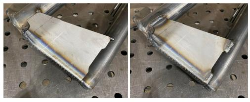
15. Weld over the tab/slot on the top surface of the top plate. Grind the weld smooth/flush with the surface.
