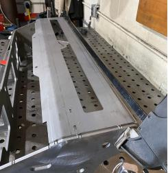
10. Take the upper cover backing plates and align them as shown. Make sure the tapped hole is up. Align the keyed edges. Once aligned, tack into place.
