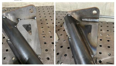
10. Fully weld around the end of the lower tube to the mounting plate.
