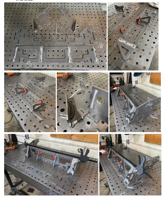
6. Make sure all tabs are fully seated and there are no gaps/angles between edges.
