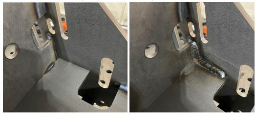
24. On the inside of the cradle, weld the top and bottom edges of the upper cover backing plate to the winch plate and formed upper cover.
