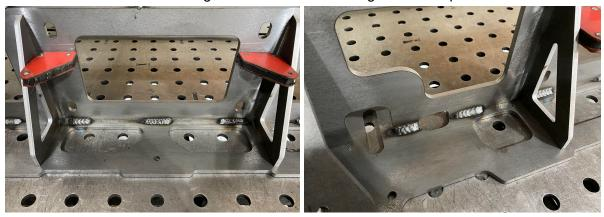
15. Fully weld the outer edges of the winch plate supports. DO NOT weld the inner edges, the weld bead could interfere with the bolts/nuts for mounting a winch.
