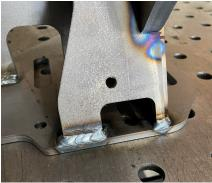
17. Weld the seam between the upper and lower cover backing plates. Keep this weld as low profile as possible to not interfere with the aluminum cover.
