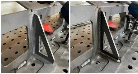
16. Weld the seam between the lower cover backing plates and bottom edge of the mounting plate.
