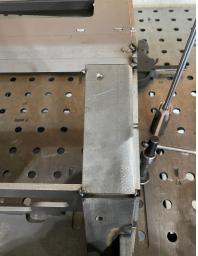
11. Take the fairlead plate and align the tapped holes on the back side of the holes on the formed upper cover. Using the provided 2x M8 flat head bolts, thread them through the cover into the holes in the fairlead plate and tighten them down. Align the bottom edge of the fairlead plate to the front edge of the winch plate. Put a few tacks between them.
