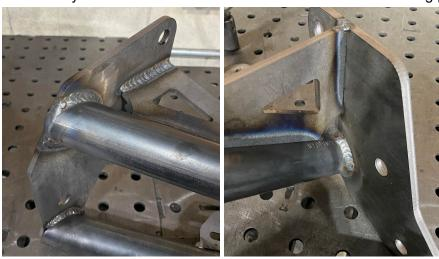
11. Fully weld around the cope where the upper and lower tubes meet.
