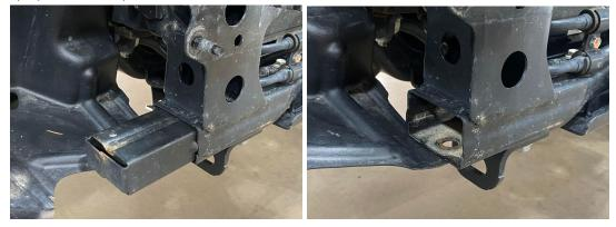
4) (OPTIONAL) If running a winch with an integrated control box that is not able to be offset to the side or remote mounted, cut out the bottom of the grille support bracket for extra clearance. Deburr and paint any cut edges.
