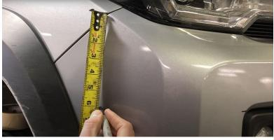
d) Mark a line 3-1/8 inches down from the same edge and parallel to the fender flare.
