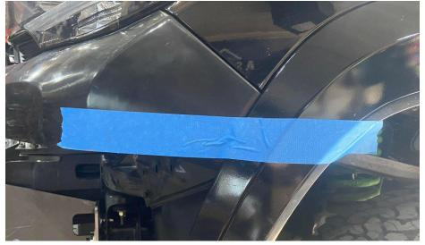
b) Using an appropriate cutting tool, cut the flares along the edge of the tape.
