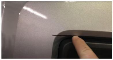
c) Mark a line 6 inches straight down from the corner where the bumper meets the fender.
