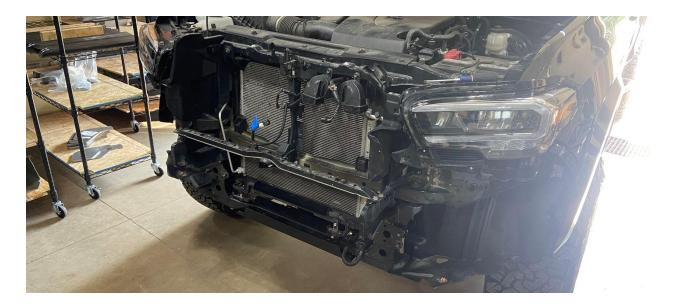
3) (OPTIONAL) Remove side crash bars from below the frame rails.
