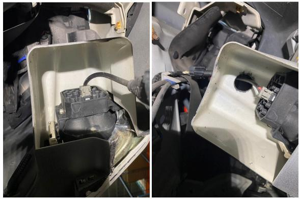
11) Cut back edges of the fog light pocket at an angle.
