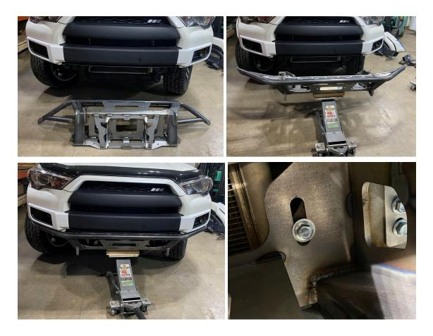
18) Install and tighten all 3x outer M10 bolts with aluminum washer plate per side.
