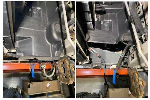
10) Drill a large hole in the top surface of the fog light pocket and reroute the fog light wiring through the hole.
