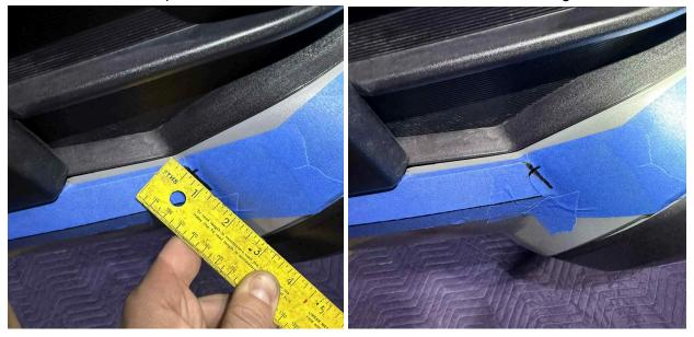
9) Trace along the body line below the fog light cutout around the sides of the bumper and to the wheel wells. Can use a laser or flexible straight edge for tracing around the sides. Make sure both sides are even by measuring down from a reference point to the line.
