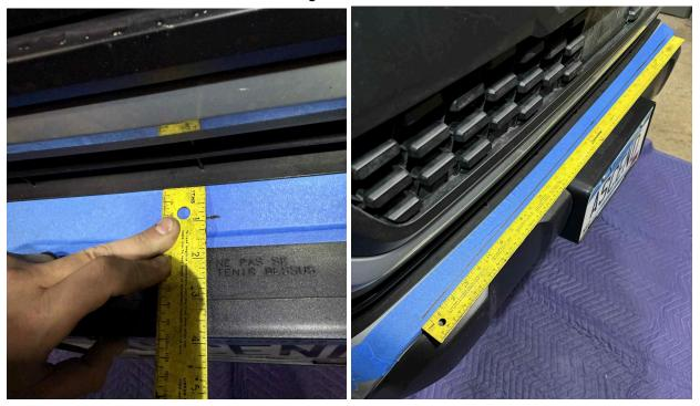
8) Trace along the valley where the surface below the fog lights meets the sloped surface at either end of the top center surface. Make a mark on it 5/8" out from the edge of the valence.
