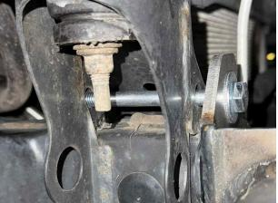
29) Put a nut and 1-1/4" OD washer on the inner mounting studs and tighten.
