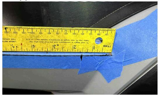
11) Draw a large arc between the mark on the line in the valley and the end of the straight line on the top center of the lip. This area will be covered so it doesn't have to be perfect. Then
