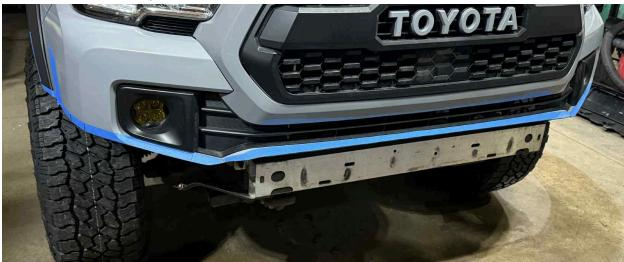
13) If using the slots on top of the bumper for mounting pods/lighbar, trim back the center edge an additional 1/2" along the entire edge or just where you plan on mounting to leave room for the hardware.
