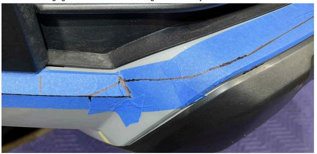
12) CAREFULLY cut along the lines. Be sure to not cut too deep behind the inner surfaces of the bumper. Recommended to apply tape over the cut areas as you go so the bumper isn't hanging while cutting. Once you finish cutting and remove the lower section of the bumper, sand/deburr the edges. Leave the tape on for now.
