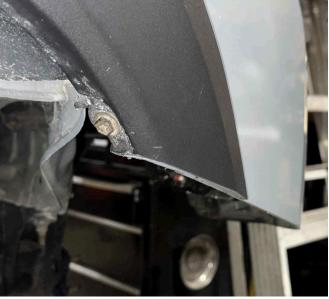
27) Install the M10\*25mm bolts with 1" OD washers through the holes and into the nut plates. Don't press too hard when initially threading it in or you might cause the nut plate to separate before you can start the bolt into it. Tighten the bolts.
