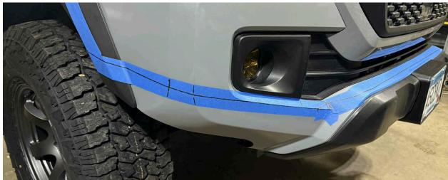
10) Measure 1-1/2" out from the line you traced in the valley and mark on the body line below the fog lights.
