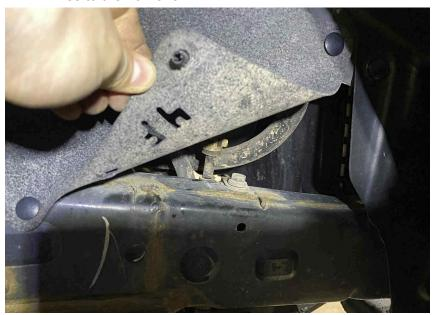
c) Loosely install the provided aluminum offset brackets. The coil feet should attach to the treaded holes on the brackets using the shorter bolts. The rest of the bracket with the slotted hole should be facing forward away from the truck.
