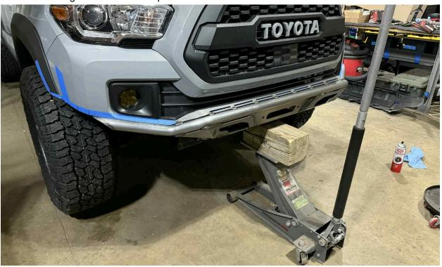
24) While holding the bumper in place, loosely install the outer M10 nuts (can use the new provided ones or reuse the oem ones) with 1-1/4" OD washers. Recheck the bumper alignment then tighten the hardware.
