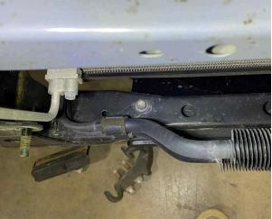
b) In the passenger side wheel well, undo the splash guard and remove the bolt holding the lines to the frame rail.
