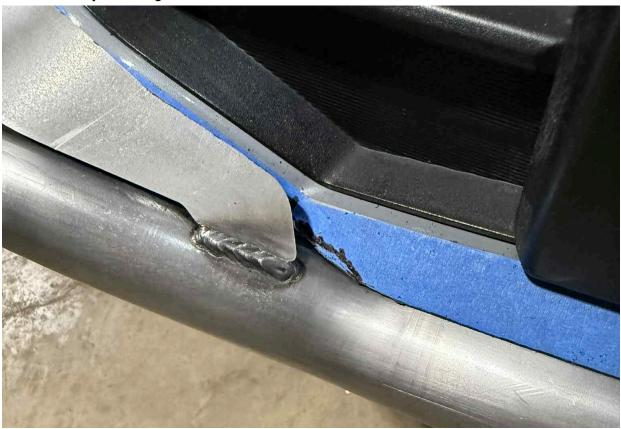
26) (OPTIONAL) If you want, can increase the side "viper" cut to a steeper angle. However it is recommended to not cut above the screw holding the fender flare on.
