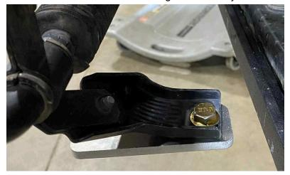
d) Attach the offset brackets to the crossmember using the longer hardware. Then tighten the shorter hardware.
