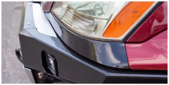
9) Once it's in the correct position, firmly press against the bottom side of the flange to fully adhere the tape to both the fillers and the headlights.
