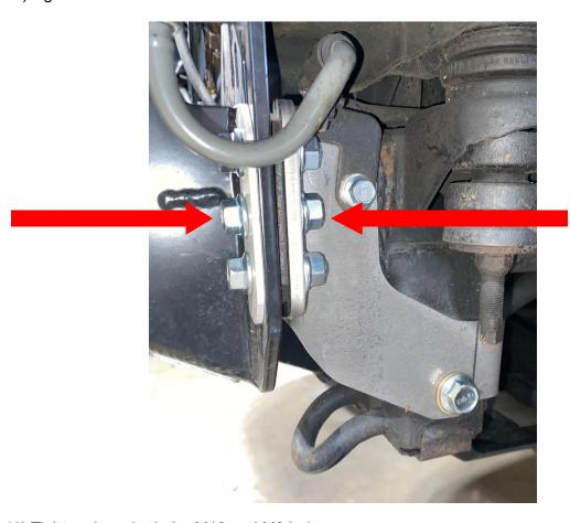
11) Tighten down both the M12 and M8 bolts.
