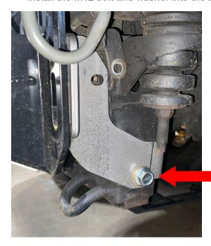
7) Loosely install the M10 bolts through the bumper, old stud holes, and frame bracket. You might have to tap or spin them through. Can be installed either direction. If running an Ascend Fab bumper, also install the aluminum washer plate.
