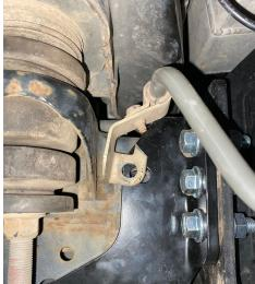
10) Tighten down M10 bolts/nuts to draw the frame bracket forward.
