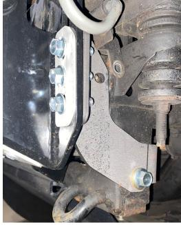
8) Loosely install the M10 nuts and washers on the ends of the M10 bolts.
