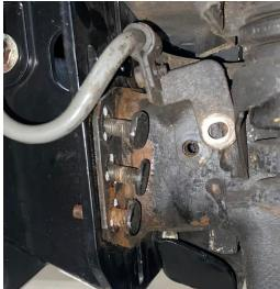
b) On models with nuts on the back side of the end plate, take one of the old bolts and install it part way into the nut on the back side. CAREFULLY hit the bolt from the side/top/bottom to break the spot welds on the nut on the back side of the end plate. You may need to use a punch rested on the bolt and hit the other end with the hammer if you can't get the hammer head in there without damaging other parts.
