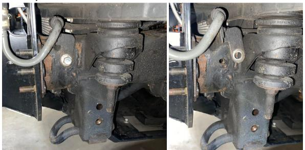
2) (OPTIONAL) Using a drill and M8x1.25 thread tap, run it through the upper holes to clean the threads of any rust/debris. Repeat this process with a M12x1.25 tap on the lower holes.
