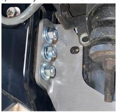
9) Loosely install M8 bolt and washer into the upper hole. If you have a hard line, first move the bracket for it over the frame bracket and install the bolt through both. You may have to trim/bend part of the bracket.
